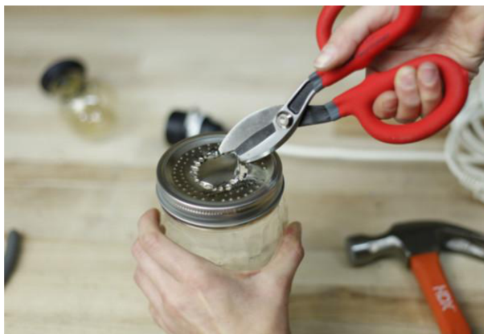
Using your tin snips, cut the rest of the center piece out.
