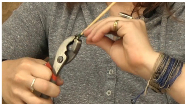
Coil the wire around a pencil or small stick so the wire has a handle.
