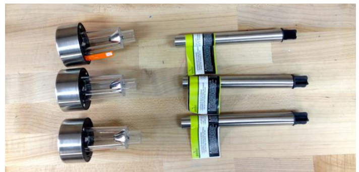
Remove the stake piece of the solar lights so you are left with the top solar panel piece.
