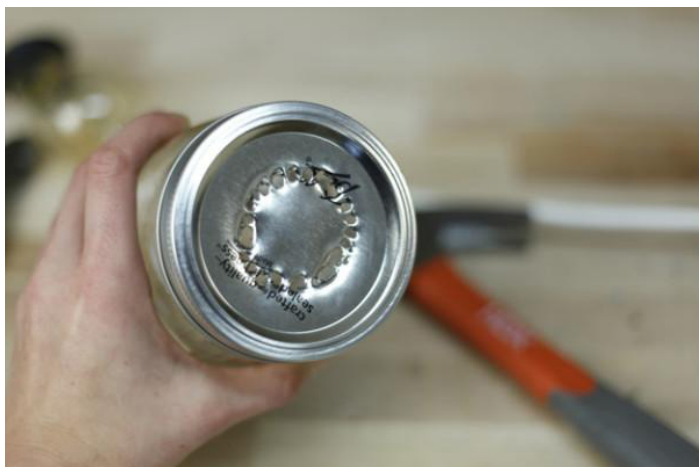
Punch holes all around the circle. The more you punch, the easier it will be to remove the center piece.
