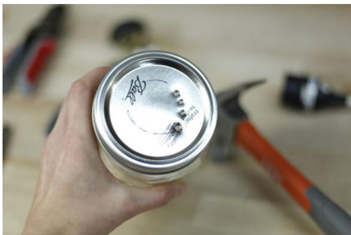
Using your nail and hammer, start punching holes along the edge of the circle.
